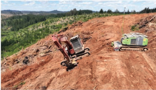
Image 2: T-winch integrated to soil preparation excavator
